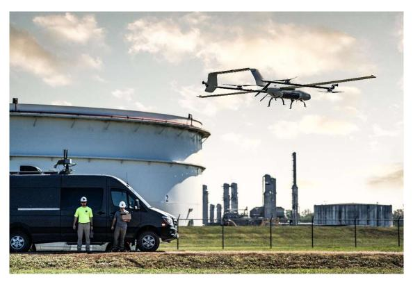
PAU with an Event 38 E455 patrolled 320 miles of Shell pipeline in under eight flight hours.
